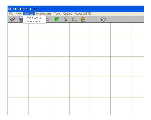
**Point source**. This is a point source. The source size is small if we compare it with the size of the area in which we are simulating (point source). If you click this button, the next dialog box is shown:
