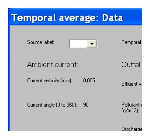
The window allows to visualize the data to make the average. It also allows to modify the data or to change them. We have two groups of data that can vary in time: Current data (velocity and angle) and Outfall data (velocity, pollutant concentration and flow rate). These are the current and discharge conditions that can vary in time in the numeric simulation.
