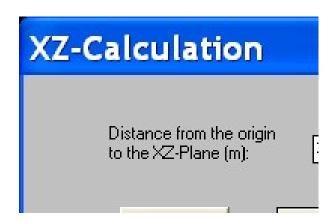
In this window we will be able to write the distance to the origin (inferior left point of the screen) of the XZ-plane that is perpendicular to the surface of the water. On this plane we will carry out the XZ-Calculation.
