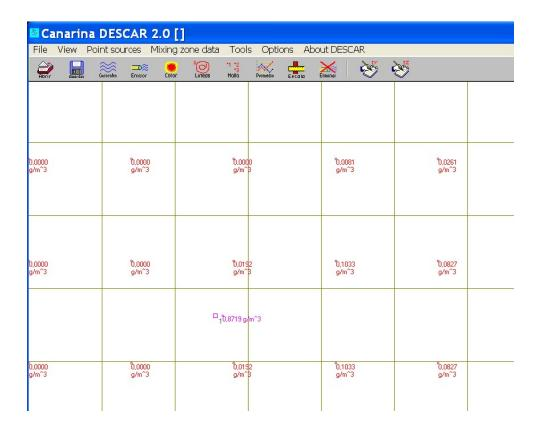
Calculation parameters. - This command will show us the parameters that we have assigned before carrying out the calculation. It is convenient their use with the purpose of verifying that we have written the parameters correctly. Once finish the calculation, the command shows us, also, the value of the maximum concentration and its position.
