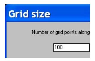
In this window we will be able to choose the number of grid points (calculation points) that we want to have in the X-Axis. The number of points to calculate will increase quadratically with the number of grid points along the X-Axis N, that is to say, it will increase as  $N^2$ .
