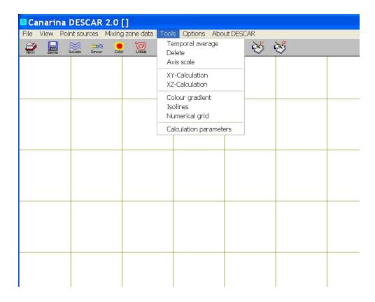
Temporal average. - Some discharge data can vary with time (velocity of the current, pollutant concentration,...). Taking this into account, the program can do temporal averages in the calculation. In the CASTOR-WATER software, these data are allowed to vary with time. If you click this command, the next dialog box is shown:
