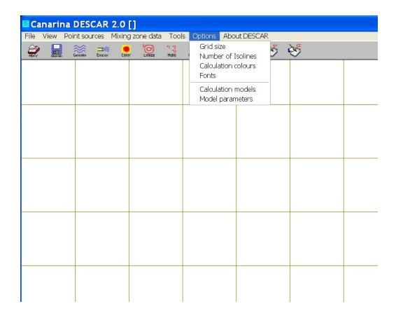
Grid size. The grid size is an important parameter in the configuration of the system. We will decide the number of calculation points in the grid that we will take to make the simulation. As we increase the number of points, the computer will take much more time in carrying out the calculation but the result will be much more exact. If you click the Grid size command, the next program window is shown:
