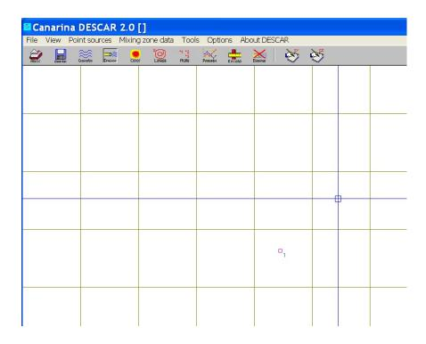
The small red square shows the outfall location. We can draw all the outfalls that we want (up to 1,000). To change the discharge data, we can click the outfall location in the program window. Then, the discharge dialogbox is again displayed. We are not able to put two outfalls in the same location. The older is eliminated automatically.
