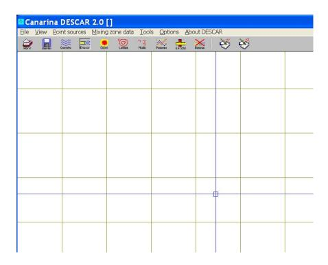
Two blue axis points the place where we can fix the outfall position. After clicking the program window, you draw the outfall.
