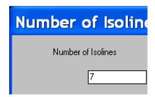
In this window we will be able to choose the number of isolines that we want to have in our computer screen. To calculate the lines, the program also considers to the maximum point as a line.
