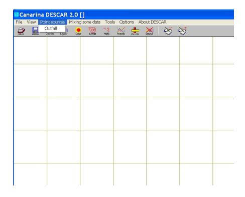
Outfall. - This is a pollutant point source. The outfall is small if we compare it with the size of the area in which we are simulating (point source). If you click this button, the next dialog box is shown:
