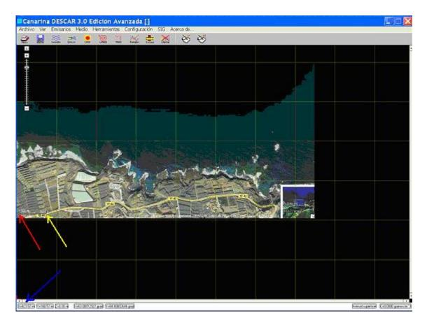
When we put the mouse pointer in the point of red arrow, it is found 7 m in the X-Coordinate box (marked with a blue arrow). If we do the same with the yellow arrow, we obtain 75 m in the box marked with a blue arrow. Then, and in our actual scale, the bar width have 75 m -7m = 68m. However, the correct value in the original Google scale is 100 m. The correcting ratio is
