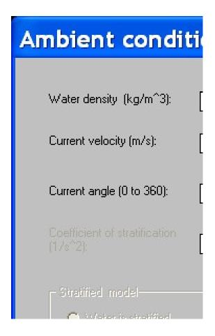
Depending on the used model, some data of the dialog box can be modified: Buoyant jet model or Stratified model (see calculation models).
